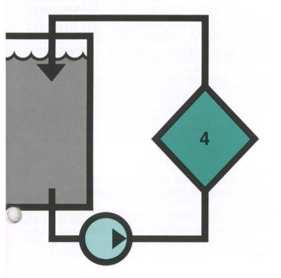
Besides providing the most efficient filtration, a recirculation loop allows other contamination-control and fluid-conditioning equipment, such as oil reclaimers or coolers, to be applied to the system. Any equipment installed on such a loop can readily be serviced without shutting down the hydraulic system.
