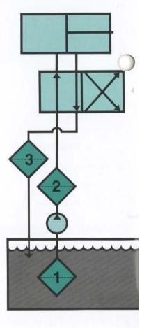
normal operation includes surges, spikes and variations in flow and pressure. Filters cannot simply be mounted in any location that offers a convenient take-off point for the fluid—a proper balance must be struck.
