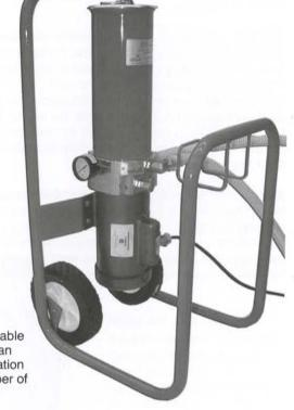
Off-line loop on wheels: A single, cost-effective portable filtration system can provide contamination control for a number of hydraulic system locations.
