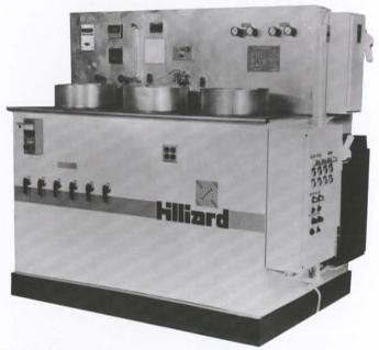
Hilliard's laboratory facilities for analysis and testing of fluids, contaminants and filtration materials includes the Multi-Pass test stand shown above, used for Beta ratio determinations (see explanation at right).
