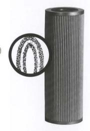
Microgard™ cartridge: A three-layer pleated cartridge, with an outer, cellulose-paper element for coarse filtration, an intermediate, glass-paper layer for microfine filtration, and an inner cellulose-paper element for added support. Nominal 0.5 micrometre rating with Beta 10 of 1000 offers excellent protection for sensitive hydraulic components, especially when used in an off-line loop.
