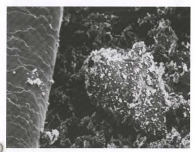
These particles, photographed under 850X magnification, are only 0.5 to 70 micrometres in diameter, but can disable a hydraulic pump or control valve. The object that resembles a tree trunk at the left of the photograph is a human hair; the object adhering to it near the bottom is about 10 micrometres in diameter.
