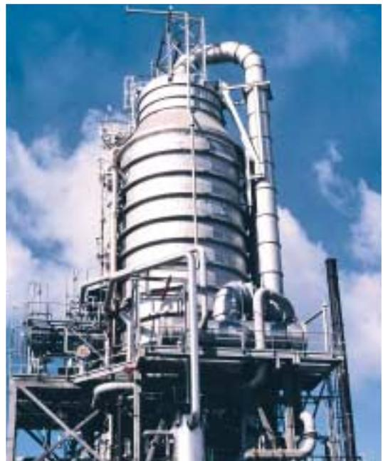
*Vacuum preconditioner on a visbreaker at a South American lube oil refinery. Vacuum system supplied as unitized system,*
