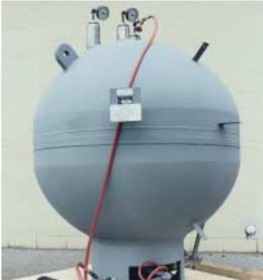
One of six large high-pressure Heliflow heat exchangers in a super-critical water treatment process.
