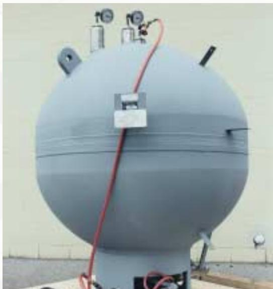
One of six large high-pressure Hellflow heat exchangers in a super-critical water treatment process.
