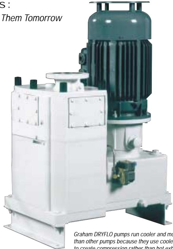
*Graham DRYFLO pumps run cooler and more efficiently than other pumps because they use cooled process gas to create compression rather than hot exhaust gas or by mechanically reducing chamber volumes.*
