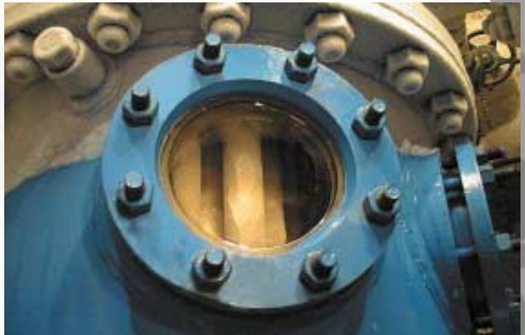
*Our freeze condensers trap and solidify product on heat transfer surfaces to improve reclamation and reduce carry-over into the downstream vacuum system.*
