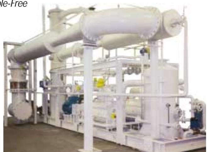
*Combination vacuum systems, commonly called hybrid systems, combine our steam jet ejectors, condensers, and liquid ring pumps for enhanced efficiency and performance.*
