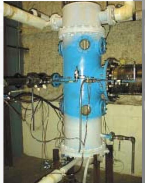
*A freeze condenser undergoing performance evaluation in the R&D facility.*
